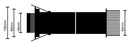
Hole size 86mm minimum, cover plate 100mm
