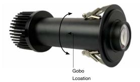
Once the front half of the unit is removed you will see where the gobo is mounted into the gobo holder, held in with a spring circlip. If there is a gobo already mounted in the light begin by removing the metal circlip which is holding the gobo in place. Swap out the gobo for your new one and do not forget to replace the metal circlip.
