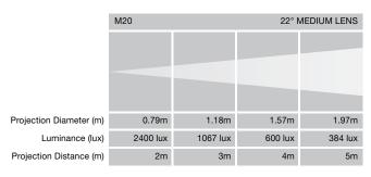
Lux values indicated are not peak values, which may be higher. We give average LUX readings taken under actual tests.
